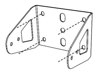
1. Hold the bracket against the wall, mark the centres of the four holes in the bracket on the wall then drill the four holes (materials not supplied). fix the bracket to the wall using suitable screws and anchors (not supplied).
