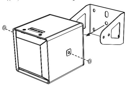
2. Align the supplied rubber washers with the two threaded inserts on the sides of the speaker.
