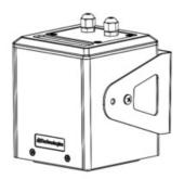
3. Fasten the speaker to the bracket using the two screws supplied in the correct position for the required tilt angle.
