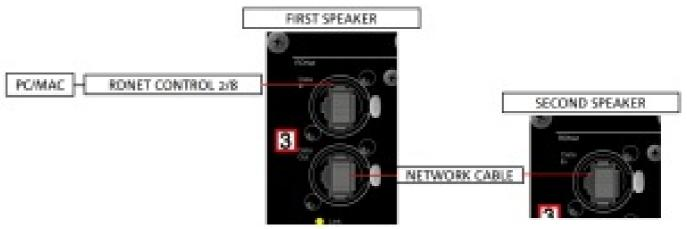
All speaker parameters can be adjusted with the remote control, once the RDNet connections have been
