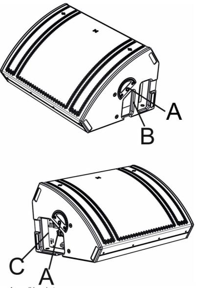
A – Mechanical housings for wall bracket
