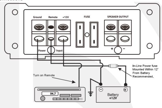
**IMPORTANT!** Before making any connections, disconnect the car's battery until the installation is completed to avoid possible damage to the electrical system.
