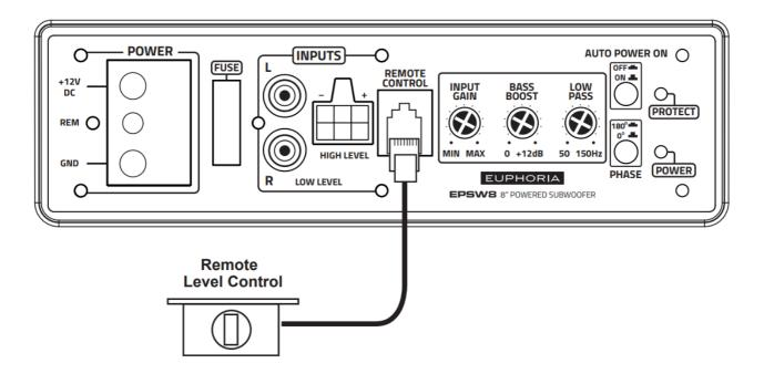
Install the remote control securely under the dash or in a similar location where using it will not distract the driver.
