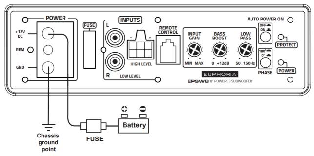
NOTE: In this connection, the AUTO POWER ON/OFF switch is in the ON position
