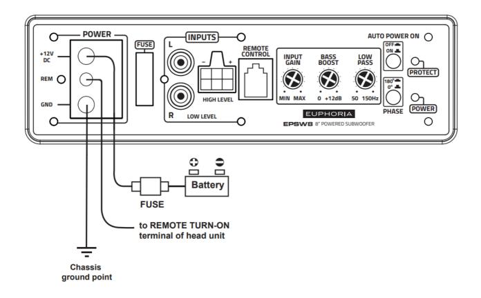
NOTE: In this connection, the AUTO POWER ON/OFF switch is in the OFF position
