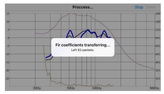
4. The image below shows an example result of a completed correction process. This measurement was completed using the linear model of correction, and three measurements averaged together for both near field and listening position. The result also used all of the settings found in previous screenshots.
