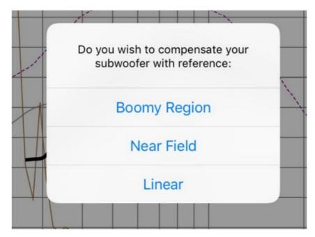
**Boomy Region** – Suitable for most types of subwoofers, this mode will retain the original 'punch' of your subwoofer but remove the most obvious and undesirable response issues from room reflections. The Boomy Region mode will correct the frequency response to fit the ideal flat line from 70 Hz and up, which is where the most annoying room reflections are likely to occur. Choose this mode if unsure of which model to use.
