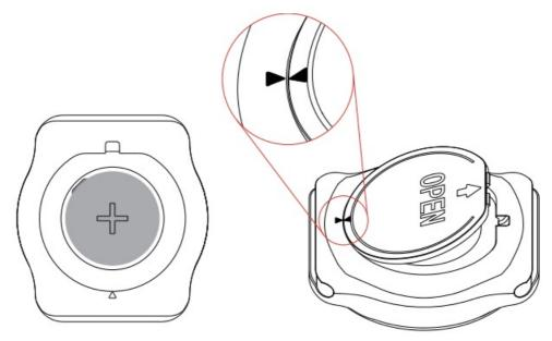
• Battery, then put the cover back to complete the battery replacement.
