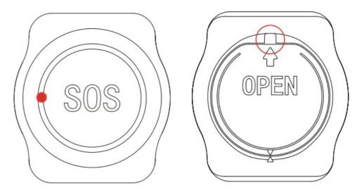
• Use a tool to lift the battery cover
