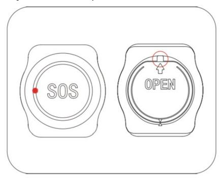
Use a tool to lift the battery cover.
