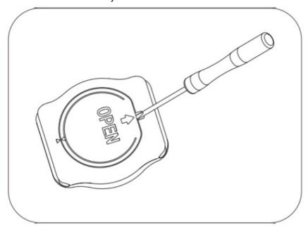
Replace the 3V CR2032 Lithium Coin Battery, then put the cover back to complete the battery replacement.
