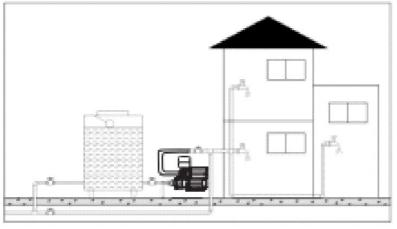
Water supply to water tank on roof and downward pressurization of water supply
