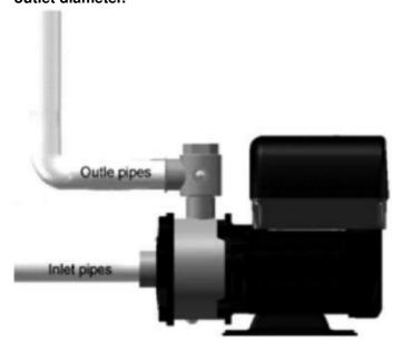
• For first time use, fill priming port with water in order to bleed air
