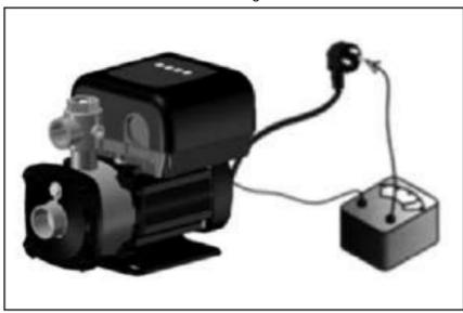
The pump should be properly installed complete with leakage protection device. The power outlet which connects to the plug should be reliably grounded.
