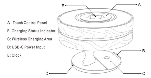
Gently touch the control panel area to set it to standby mode when control icons are lightened. It will be in sleep mode if no operation in 30 seconds and control icons are off.
