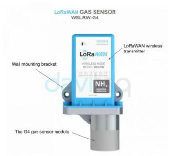
The G4 gas sensor module measures the gas concentration in the surrounding environment. The LoRaWAN wireless transmitter is to read the measurement values from the G4 sensor and performs the scaling and calculation to deliver the desired output values, then it sends data to the gateway in the following cases:
