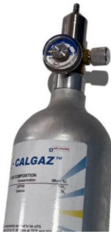
Step 3. Installed the Regulator to the Gas cylinder
