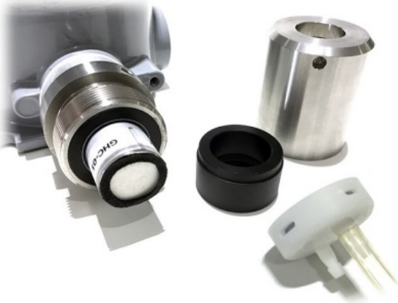
Step 1. Remove the Filter and prepare the calibration cap
