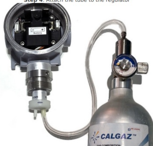
Step 4. Attach the tube to the regulator
