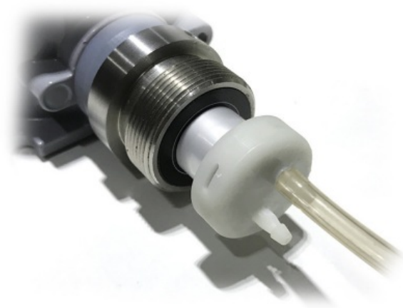
Step 2. Attach the calibration cap to the sensor head
