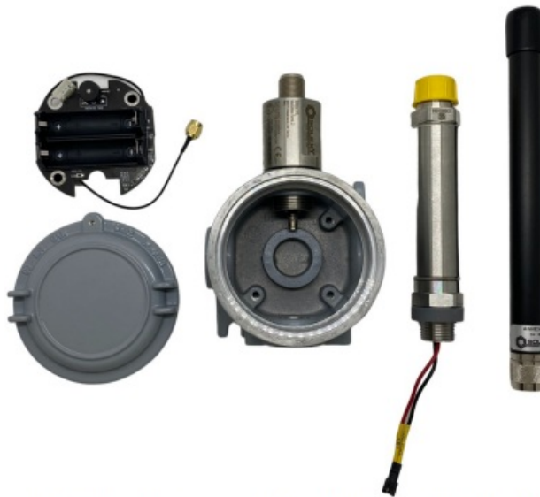
Figure 2.7: Components of Daviteq Sigfox Exd Pressure device after disassembly.
