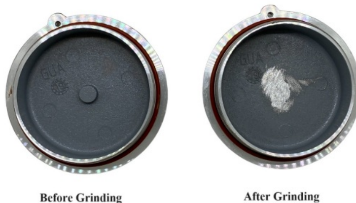
Figure 2.2: Grind the excess part inside the housina cover.
