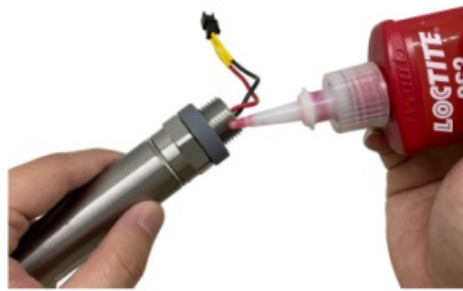
Figure 3.1: Apply thread lock glue to the connection thread of sensor.
