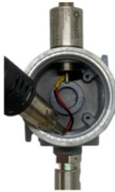
Figure 2.5: Heat up the connecting thread.
