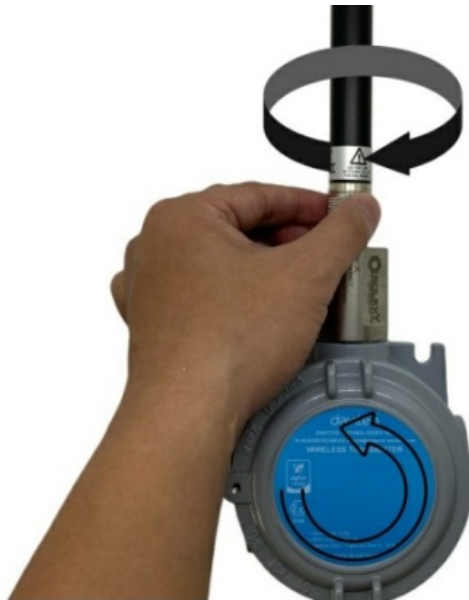
Figure 2.1: Unscrew the antenna and open the housing cover of Daviteq Sigfox Exd Pressure device.
