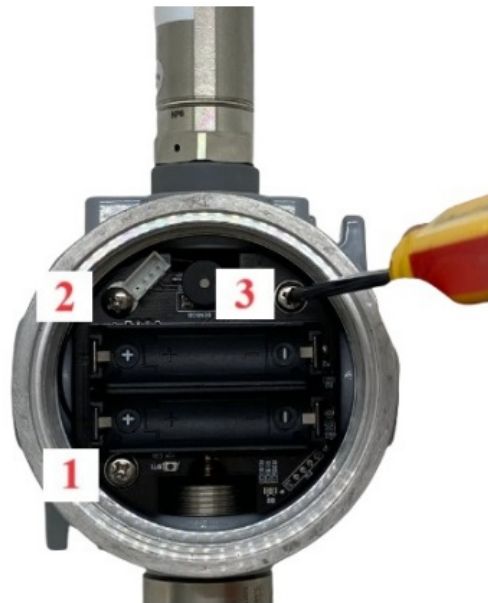
Figure 2.3: Remove the Sigfox mainboard by screwdriver.
