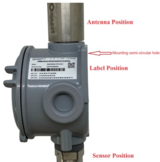
Figure 4.2: Position and direction of the device information label on the housing
