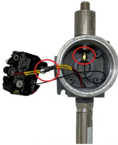
Screw the antenna cable and plug socket of sensor cable.
