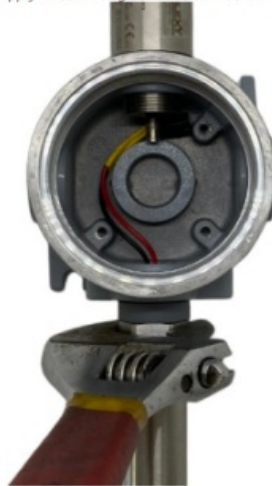
Figure 3.2: Screw the sensor to the housing by turning clockwise using wrench
