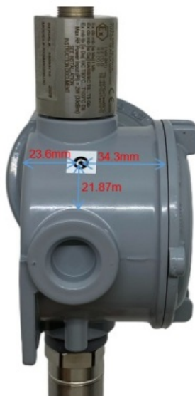
Figure 4.3: Position of the magnet reed-switch label on the housing
