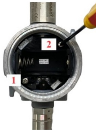
Figure 3.4: Position of 2 screws on to screw the LoraWan mainboard to the housing.
