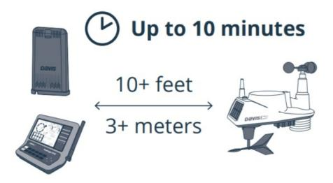
**Note:** For best reception during this step, WeatherLink Live and/or Console and the Sensor Suite should be at least 10 feet (3 meters) apart. (Initial reception typically takes 1-3 minutes but can take up to 10 minutes depending on specific environmental conditions.)
