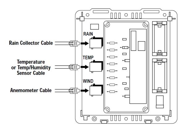
• Gather the sensor cables and secure them to the cable tie lug using a cable tie. When tightening the cable tie, make sure the cables are on top of the lug.
