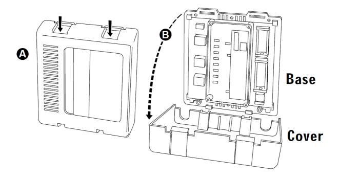
Attach the base to the mounting surface using the #6 x 1" screws.
