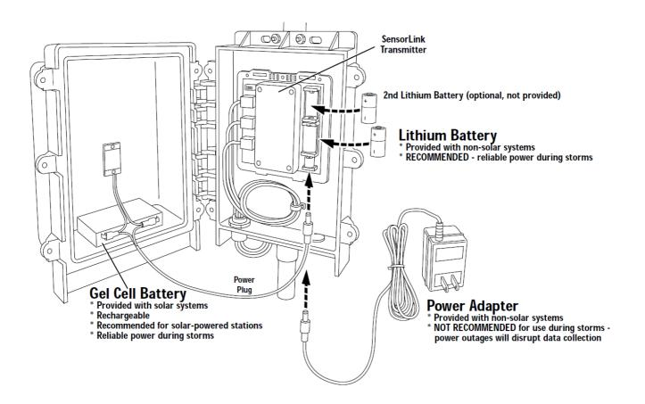
Note: This illustration (as well as the following one) shows the transmitter mounted inside a Davis Multi-Purpose Shelter (#7728). The Multi-Purpose Shelter is not required, but the transmitter does need to be mounted in weatherproof location.
