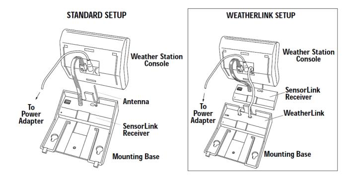
When you apply power to the console, the console should beep three times within 20 seconds to indicate that the console and receiver are working properly (or 4 times within 30 seconds, with the optional Weather Link).
