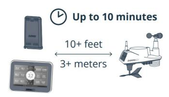
Verify data transmission from the Sensor Suite to the Weather Link app or to the Console.
