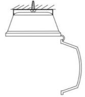
5. Detach gear tray by loosening the four retaining screws and sliding out of place. Ensure lanyards are hooked into the gear tray for safety.
