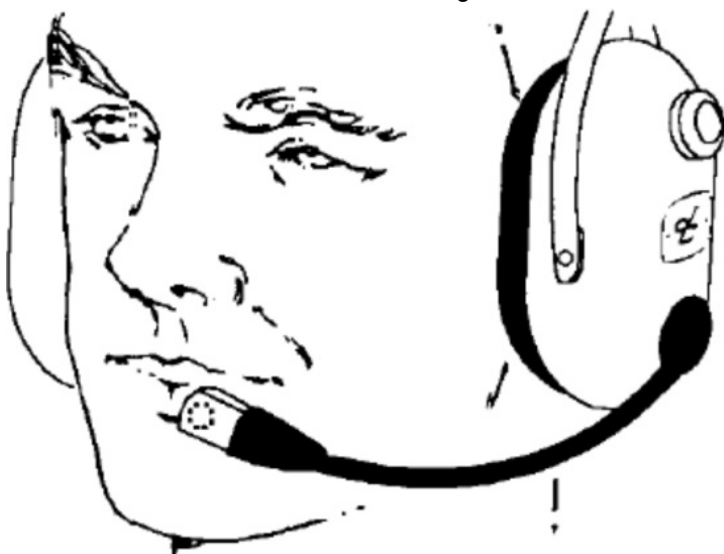
Figure 3: Microphone, Proper Position
