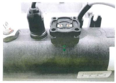
19. Place the screws into the retaining plate and evenly tighten them down. Tighten the screws in a cross pattern to achieve this
