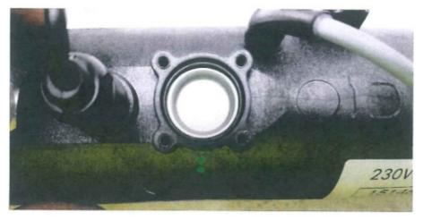
17. Place O-ring 1 onto the retaining plate. Make sure that it is not twisted and is sitting flat. Fit the thermal overload into the retaining plate. As the plate is molded to the thermal overload shape the thermal overload only goes in one way.
