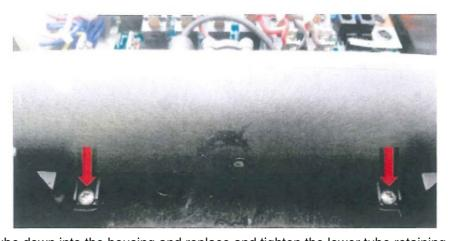
23. Slide and sit the tube down into the housing and replace and tighten the lower tube retaining screws and the upper tube retaining screw.
