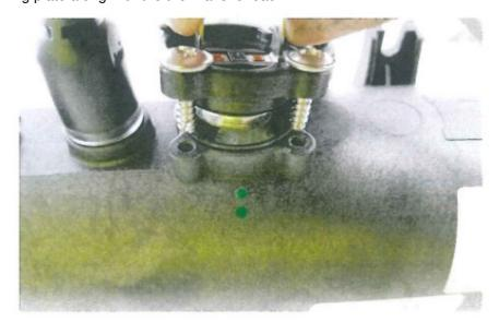
11. Now the thermal overload cup can be seen. Remove the O-ring that sits between the retaining plate and this cup. Gently lift the cup using the Small Flat Blade Terminal Screw Driver and remove.
