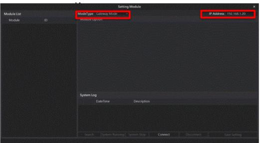
7. Click on "Connect"Note: The IP address must be in the same domain as the MELSEC-Q controller
