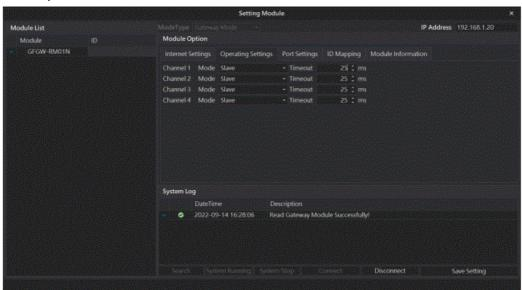
**Note:** Set Group 1 as Slave and set the gateway to use the first set of RS485 port to connect to the main controller (GFMS-RM01N)
