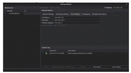
Note: The IP address must be in the same domain as the MELSEC-Q controller
