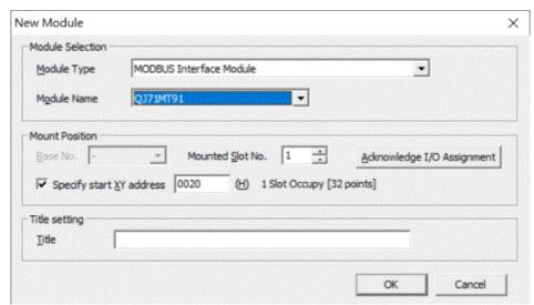
2. Launch GX Works 2 and select the "Intelligent Function Module" menu under "Project" on the left side. Then click on "Switch Setting" in the "QJ71MT91" menu
