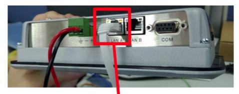
II. Connect the port at the botton of the machine to the gateway's port
