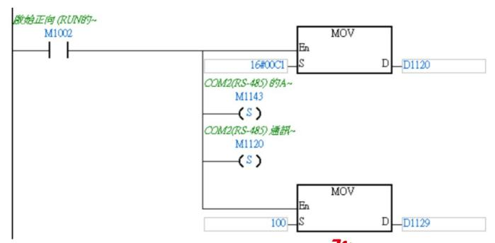
\*The communication parameter setting must be consistent with in-GRID\*\* to enable communication II. Use the MODRW command to setup the reading/writing of in-GRID\*\* is I/O module
