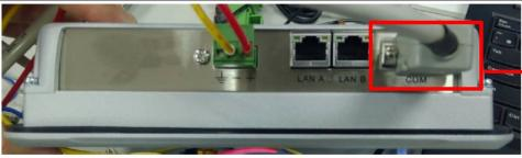
II. Connect the COM (RS485 A/B) at the bottom of the machine to the interface module (1/2) to convert it into a RJ45 connector, which will be connected to the main controller
