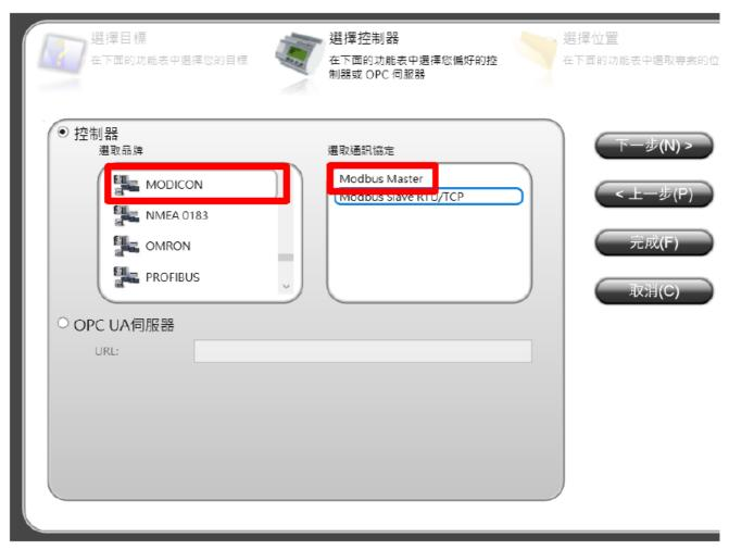
2. Click on the "Controller" tab to enter the controller setup page. Select the controller and then click on "Settings"
