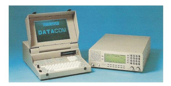
A complete 125-watt HF base station for voice or multi-mode (RTTY, CW, ARQ and Packet) data transmission. The system includes a transceiver, AC power supply, TW9200 Datacom Terminal, ASS broadband antenna, cables and microphone. It is also available with AT7000 automatic antenna tuner for use with whip and wire antennas.
