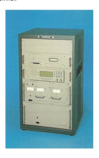
A complete 1000-watt HF base station that is mounted in a rack cabinet and includes a transceiver, 1-kW amplifier, power supply, antenna tuner (not shown), 10m whip antenna, cables and desk microphone. The system is also available with an ASS broadband antenna.
