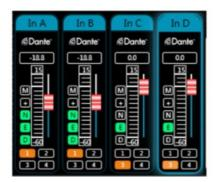
User can quickly set channels in groups for opening or closing mute, phase, noise gate, PEQ and delay function.
