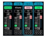
There are 3 kinds of input signal in some products: ANALOG, DANTE network audio, testing signal and AutoMix (analog and Dante). It will show a label for user.
