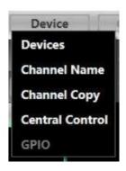
**Devices**: view or modify the software version information, device name and device IP address of the upper and lower computer of the device. Set password of device.
