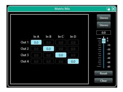
In the above figure, input channel (on top side) corresponds to output channel. The value box with a value is mixing key of channels. When the mixing key is green (double-click the value box to switch the state), the input channel and output channel signal realizes the mixing function.
