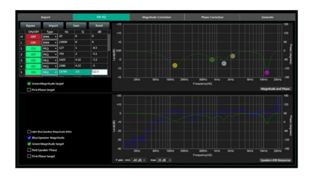
There are High pass filter and low pass filter for setting frequency divider, and 15 bands of PEQ LSLV HSLV to adjust magnitude. Try to set a linear magnitude of target speaker. Mark: changing FIR magnitude doesn't effect its phase.
