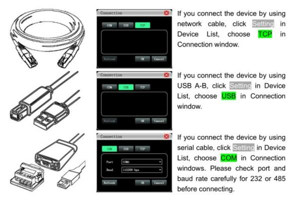
The software will use the method set last time to check if the device is connected. If successfully connected, devices will be shown in device list.
