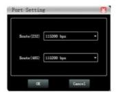
**Port**: set the connection mode, port number and baud rate, confirm the connection mode and then select the corresponding port.
