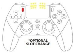
3. Press & hold the SHARE button while also holding the FUNCTION R paddle you wish to assign to, the lights will start to flash quickly in BLUE, now release buttons.
