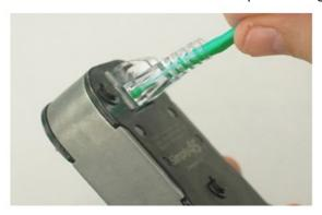
**STEP 14**Make sure plug goes completely inside the crimping socket.
