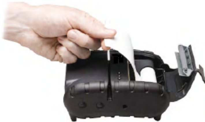
FIGURE 7: OPERATOR CONTROLS AND PAPER LOADING
