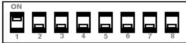
FIGURE 10: DIP SWITCH SETTINGS (SHOWING SETTING FOR IRDA)
