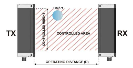
The beam interruption due to the passage of an object inside the controlled area caused the closing of the switching output and the variation of the device analogue output signal. Small objects can be detected (reaching dimensions of only 5 mm) and determine linear measurements with a 3 mm error in best cases.
