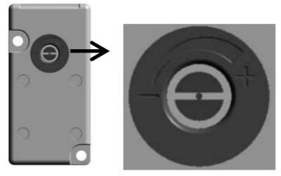
Rotate the trimmer clockwise to the limit (maximum emission), then align RX and TX at the required operating distance (LED OUT off); decrease emission power rotating the trimmer counterclockwise until the output switches (LED OUT off) or the limit is reached (minimum emission); in the first case, rotate the trimmer clockwise until the output switches again and LED OUT remains off.
