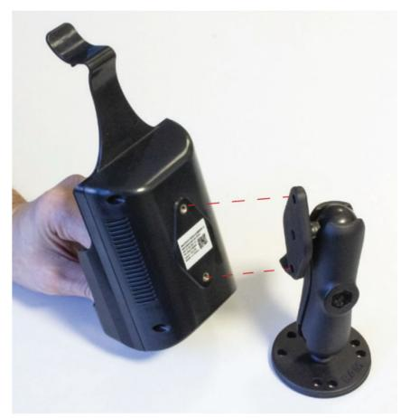
2. Secure the adjustable arm to the rear of the dock using two screws M5X10 and two nuts M5:
