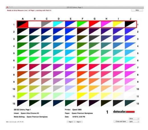
This is the window that opens whenever you're going to measure patches from target prints. What you're seeing is a grid of color patch "slots" that corresponds to the physical patches printed in the Target you chose. The grid is labelled in columns by letter, and in rows by number, to also correspond to the physical target print. The bold "1" in
