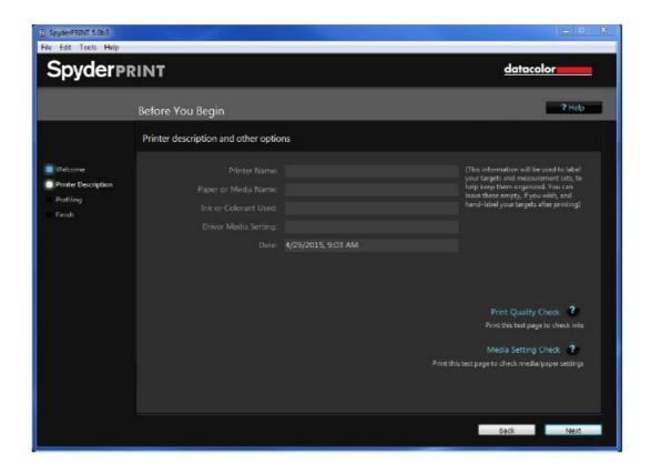
Here you can enter the name of your printer, type of paper and ink used and any driver media settings you may be using. This information will be printed automatically at the bottom of the profiling "target" sheets to help keep track of the settings that you will eventually use when actually printing the target sheets. It is not necessary to fill in all of the fields, but can be useful down the road.
