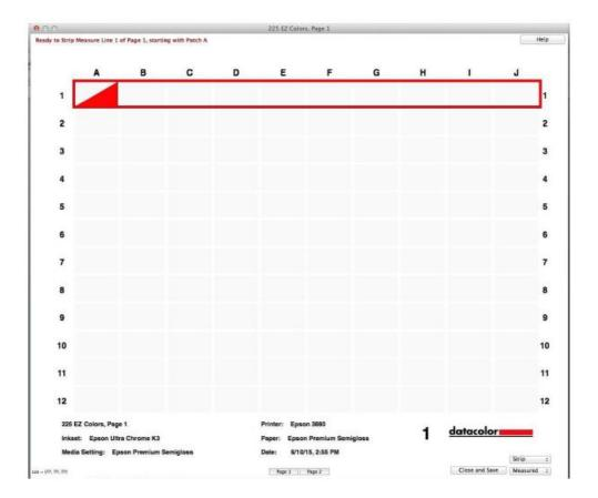
If you switch display mode to "Measured", then all of the rectangles in the Target window are filled only with the measured color. Here, this means that the entire window appears with "empty" white patches because nothing has been measured yet.
