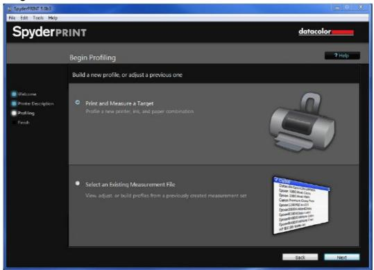
On this screen you will select whether to print and measure a Target or Select an existing measurement. Click "Print and Measure a Target" to create a new profile.
