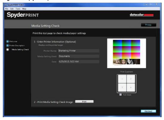
This screen lets you print a "Media Setting Check" image at different driver media settings (paper type, output resolution, etc.) to assure that the media setting choice is optimal before printing a full profiling target for the printer. If the choice is not optimal, then the resulting profile will not have the color range or detail it would have from an optimal setting, and it's likely that prints with these settings will have various kinds of cosmetic issues.
