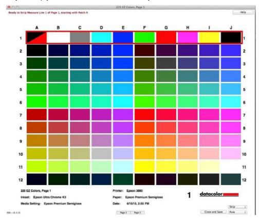
If you switch display mode to "Pure", the entire window will redraw showing all patch rectangles filled fully with the Pure colors. This will let you quickly see what the Pure representation of the target print looks like.
