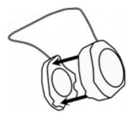
Hang the SpyderX unit over your display when asked, using the lens cap, which slides on the USB cable, as a counterweight to keep it in place. If necessary, angle your display back to keep the SpyderX flat against your screen.
