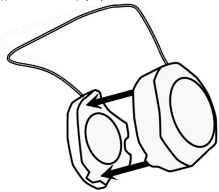
Hang the Spyder unit over your display when asked, using the lens cap, which slides on the USB cable, as a counterweight to keep it in place. If necessary, angle your display back to keep the Spyder flat against your screen.
