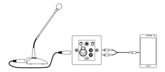
Other possibility would be using the minijack input connector for the line input.
