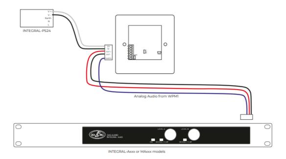
The INTEGRAL-WPM1 needs to be connected to an external 12-24Vdc power sup-ply. DAS Audio's INTEGRAL-PS24 with uni-versal mains is ideal to be installed inside walls and construction structures.
