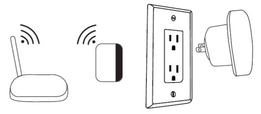
2. Search the WiFi network on your device named "wifi repeater-xxxxxx", then connect to the extender network. If you can't find the extender, reset the extender by using a pin to press the reset button and try again.
