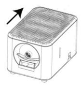
2. Pull out the plug and add the bubble liquid into the compartment.
