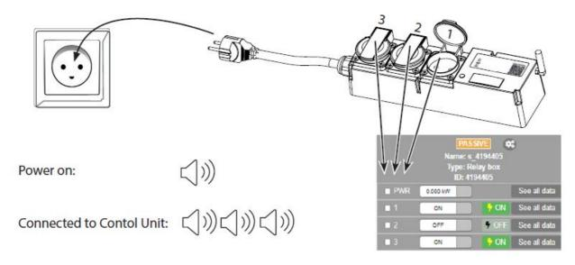
Various equipment can be connected to the Relay Box
