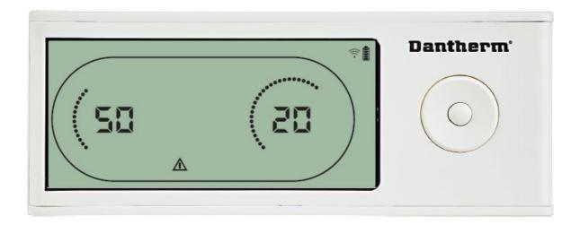
If the dehumidifier enters fail mode, the warning sign () will be shown in the DRC1 display.
