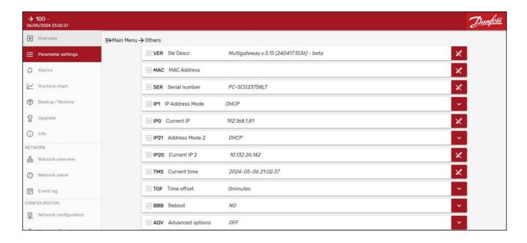
• In the case of STATIC IP management, set up parameters IP1 & IP21 to "Static". BBB parameter can be used in case of a manual reboot of the X-Gate machine.
