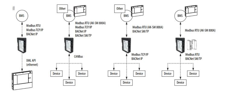
X-Gate can provide flexibility with a focus on 3rd party device integration into System Manager and at the same time make it easy for a BMS to integrate the desired data points over standard protocols.
