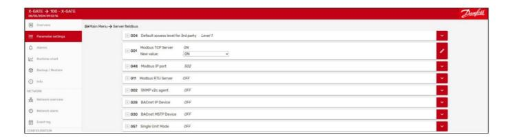
In case of sharing data with a local BMS, the full list of variable/data-points can be downloaded as a CVS file with the utility in settings download CSV file.
