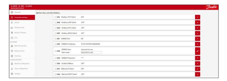
After this configuration done, X-Gate will start to automatically collect data from the System Manager and automatically will create all the CDF files of the discovered devices (nodes) and create the related device in the Network Configuration page. As a step 2, User must activate the "Destination of the data", in this case Modbus TCP/IP. In this case the activities to be done are the same already described for the Use Case 1 to set up the destination of the data.
