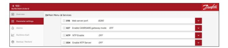
Parameter NTP will enable X-Gate to synchronize the time with an online service. Parameter G54 will enable X-Gate as an NTP Server for another Client.
