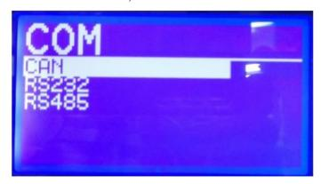
Back in the BIOS menu: Press the down arrow to access the CAN settings. These settings control various aspects of CAN communication: Node ID, Baud Rate, Active Nodes, Diagnostics, and LSS.
