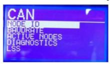
• In Node ID you can select the CAN address for the display itself which is as default 126. In Baud rate we need to select 50K:
