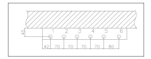
The pipe placement can deviate from the shown drawing. Please note the markings on the station.
