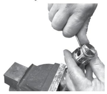
7. Remove the O-ring at the thread end of the valve with a small screw driver.
