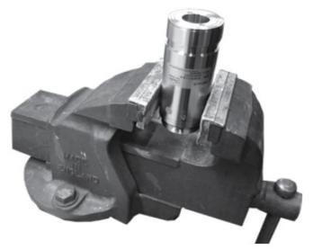
2. Turn the nut CCW with snap ring pliers.
