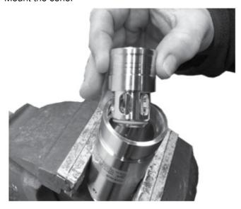
5. Mount the spring onto the cone.
