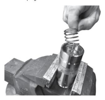
5. Remove the valve cone.
