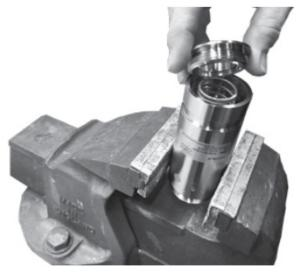
8. Tighten the nut with a snap ring pliers.
