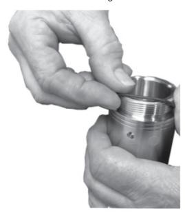
3. Mount the water lubricated O-ring on the cone. Ensure the O-ring is pushed fully into the O-ring groove.
