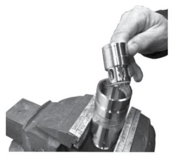
6. Remove the O-ring at the cone with a small screw driver.
