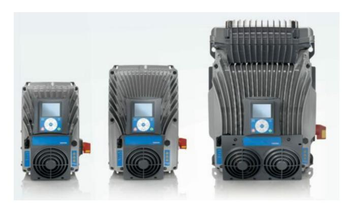
With a power range from 1.1 kW to 37 kW the VACON® 100 X sets a new benchmark for decentral drives. It comes with IP66/Type 4X outdoor protection rating and has highly advanced control capability which guarantees processes run exactly how you want them to. On top of all this, it has built-in harmonic filtering chokes, making it suitable for public networks.
