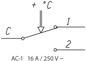
AC-1 16 A / 250 V ~ AC-3 7.5 A / 250 V ~ AC-15 1 A / 250 V ~
