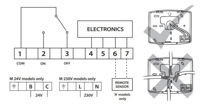
**Note:** 1.0 mm2 solid copper cable should be used to connect the remote sensor to the TP7000A. Please ensure that:
