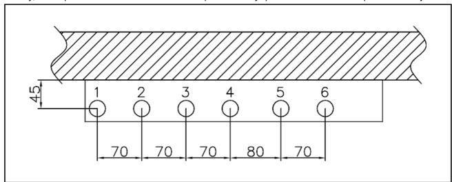
The pipe placement can deviate from the shown drawing. Please note the markings on the station.
