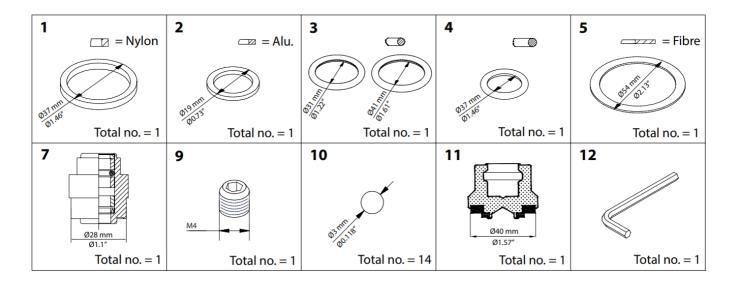
**NOTE**: When replacing the packing gland (pos. 7) in SVA-S/L, SVA-ST/LT or SVA-HS the aluminium gasket (pos. 2) is needed.
