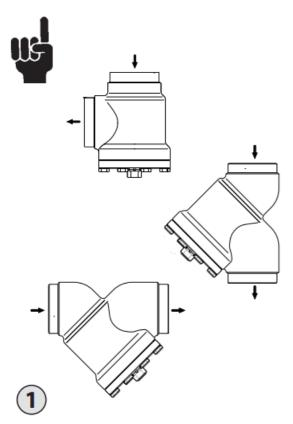
The strainer housing is designed to withstand a high internal pressure. However, the piping system should be designed to avoid liquid traps and reduce the risk of hydraulic pressure caused by thermal expansion. It must be ensured that the strainer is protected from pressure transients like "liquid hammer" in the system.
