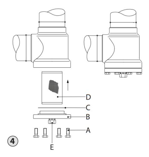
Before servicing the strainer, isolate it from the system. Drain CO<sub>2</sub> e.g. via the top cover connection to above 5,2 bara to prevent large formation of dry ice before evacuation to zero pressure. Check for refrigerant pressure before unscrewing and removing the top cover. The strainer insert must be removed without any use of tools.
