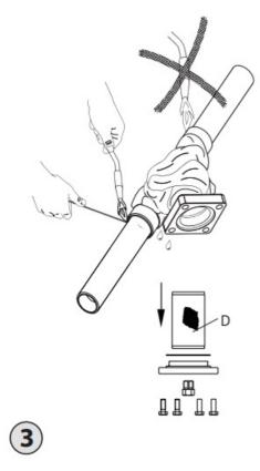
If the drain valve has been chosen as accessory, the drain plug should be replaced by the drain valve.
