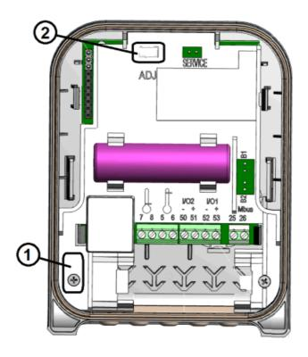
**NOTE:** With the removed ADJ protective cover. The Manufacturer warranty is void!!! **Meter calibration/ adjustment mode (continuous)**
