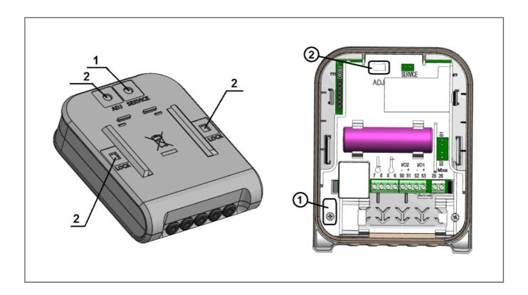
By short-circuiting the contacts "SERVICE", the SERVICE mode is activated, symbol "<->" and sign "TEST" are displayed on the LCD.
