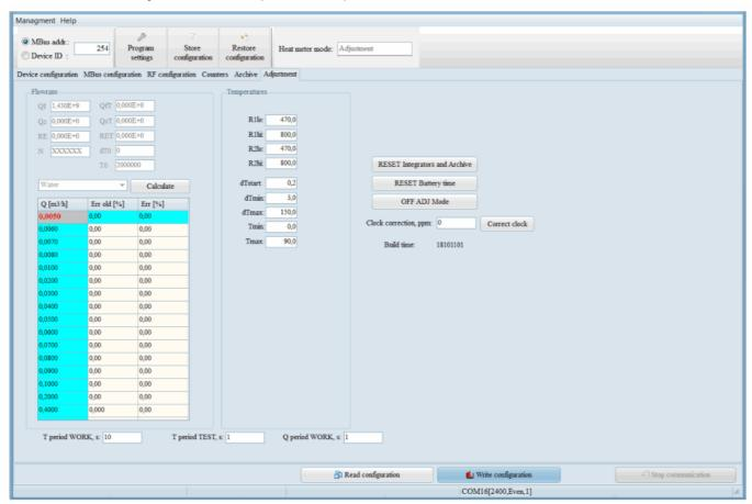
**RESET Integrators and Loggers** – intended to reset the integrator and logger values to a zero.
