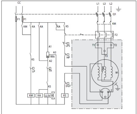
SH 180 SM 115 - 125 - 160 - 175 - 185 SZ 115 - 125 - 160 - 175 - 185 versions with electronic module This Danfoss scroll compressors compressor motor is protected by an external module protecting against overheating and high current draw.
